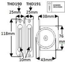
Case Material: Galvanised Steel Faceplate Material: Brass Plate Weight: 160 grams inc screws Size of Plate: 118mm x 25mm Depth of Product: 34mm
